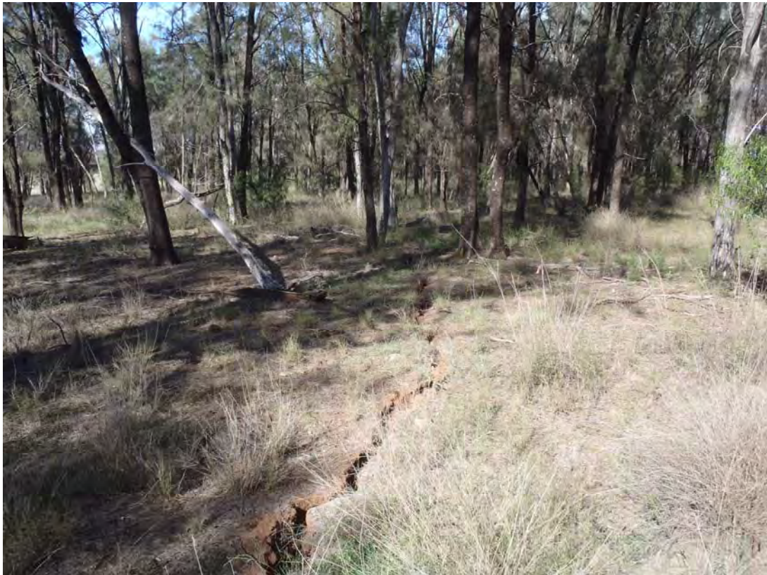
Photo 3: Surface Crack in LW102
